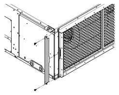
Slowly pull out the air filter (composed of 3 equal parts).
