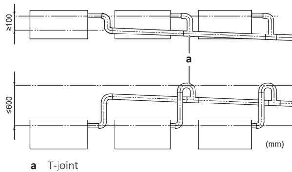
**To connect the drain piping to the indoor unit**
