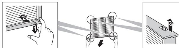
**4** Clean the suction grille. Wash with a soft bristle brush, and water or neutral detergent. If the suction grille is very dirty, use a typical kitchen cleaner, leave it on for 10 min, then wash it with water.
