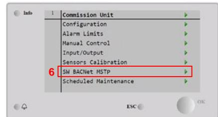
7. Select proper parameters for BACNet MSTP communication
