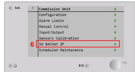
7. Select proper parameters for BACNet IP communication
