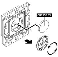
The battery is already installed on delivery. Battery life in normal use: 3 to 5 years  $\,$
